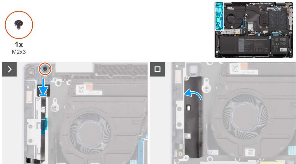
Figure 36. Installing the power button with fingerprint reader
