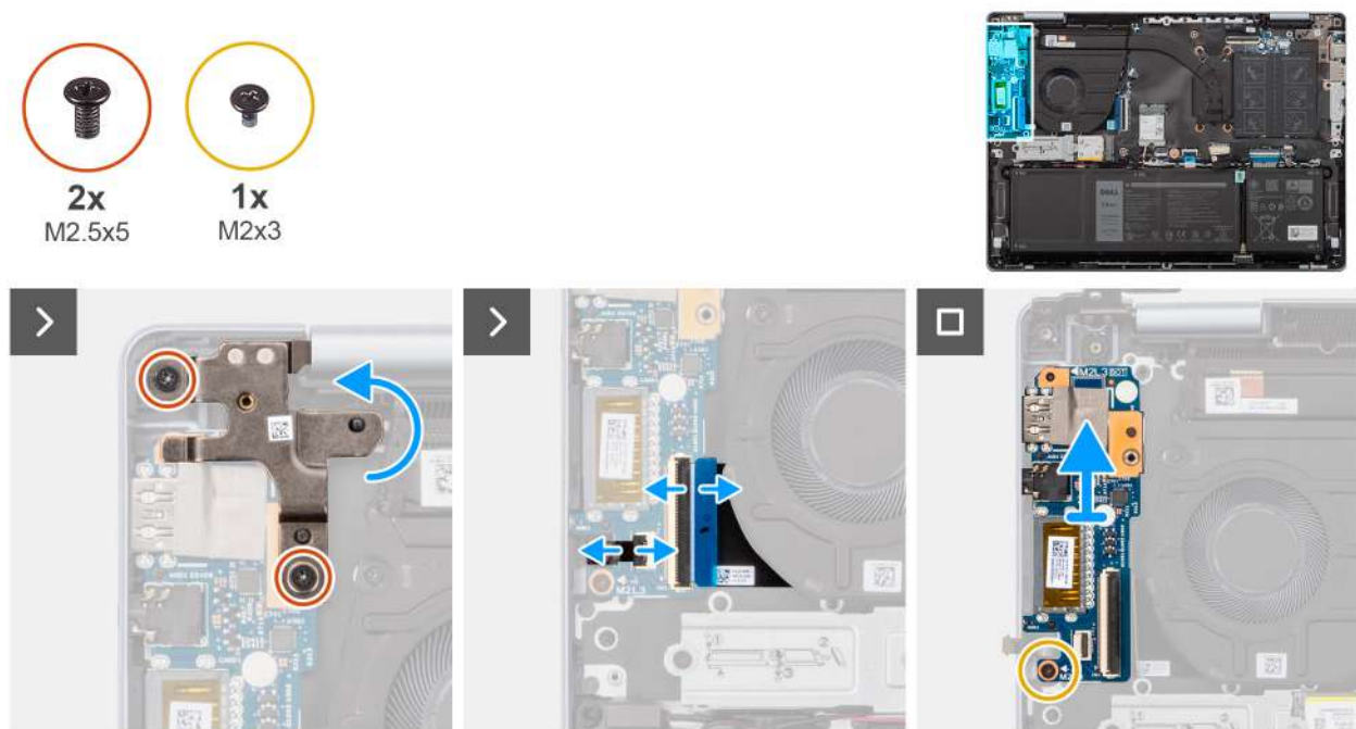
Figure 31. Removing the I/O board
